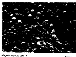
Scanning Electron Microscope Photograph of a dried Alumina Dispersion (10% Al 2 O 3 )
