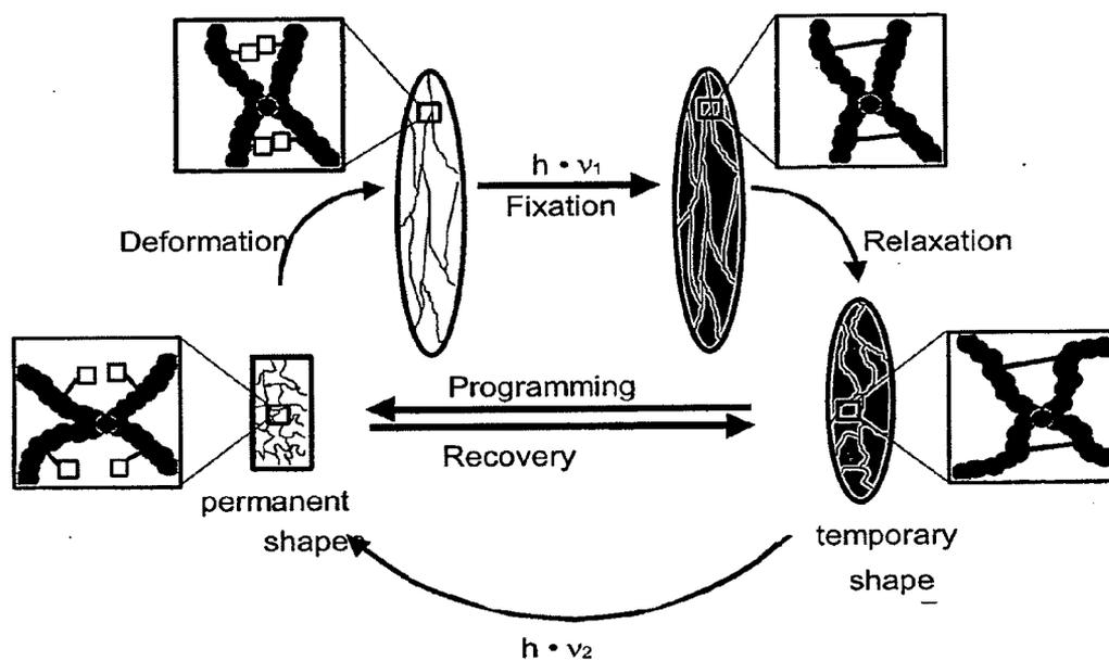
Functional principle of a photosensitive network on the macroscopic and molecular level
