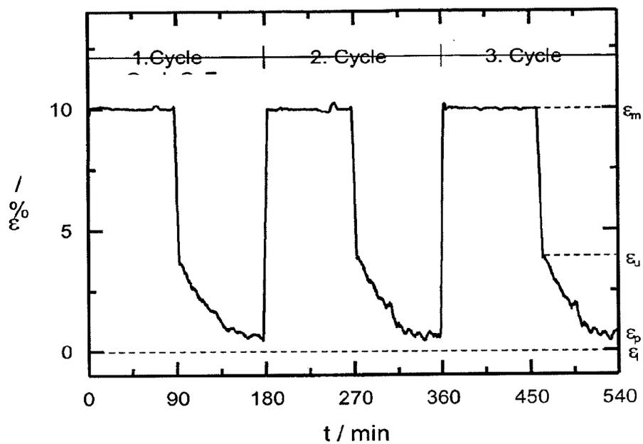
Elongation  $\epsilon$  of a photosensitive network (Sample 7A) during 3 repetitions of a photomechanical cycle (stress regulated)
