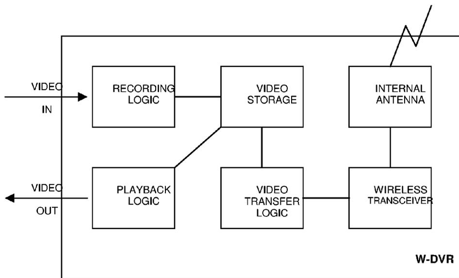
FIG. 1: Block Diagram of a DVR with Internal Wireless Transceiver
