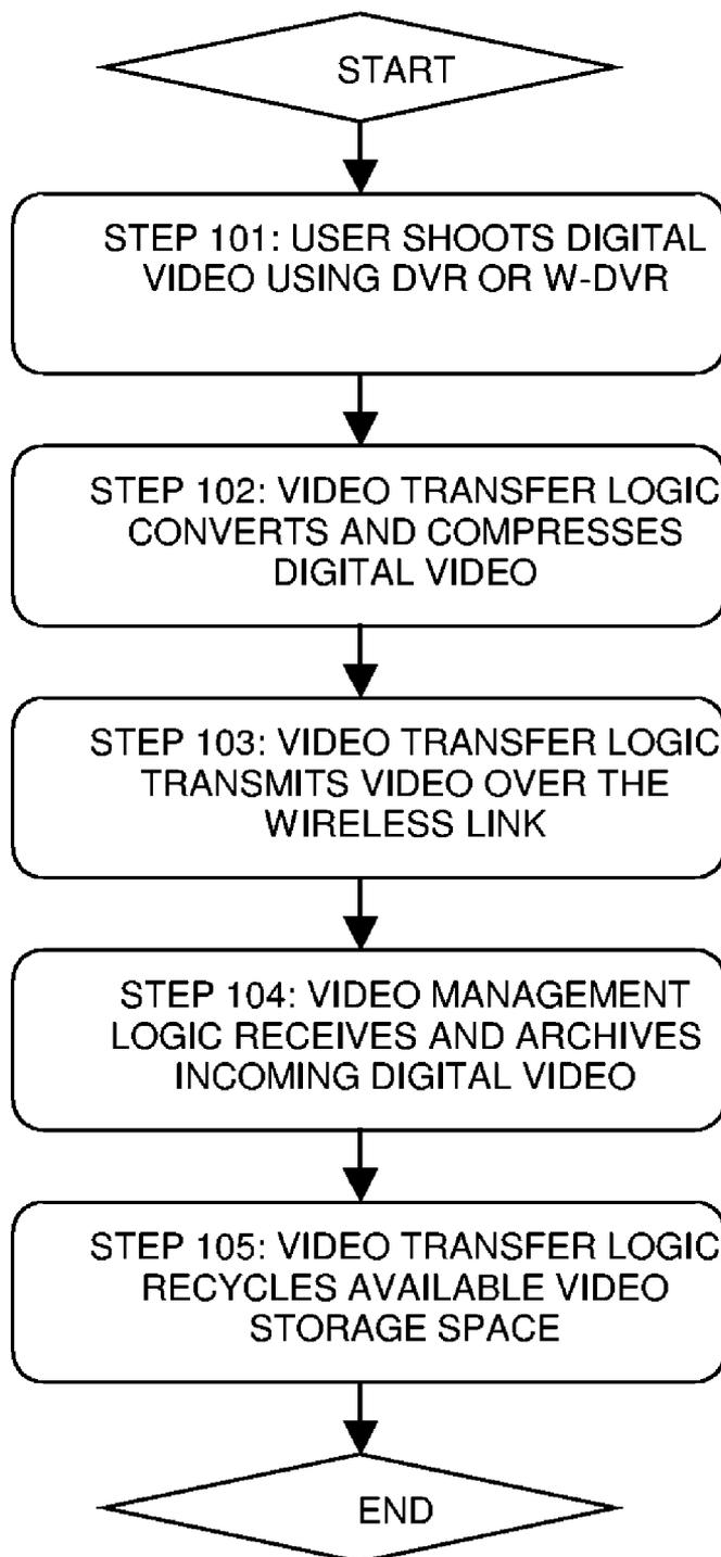
FIG. 4: Flow Diagram for to Transfer Digital Video over a Wireless Communication Link.
