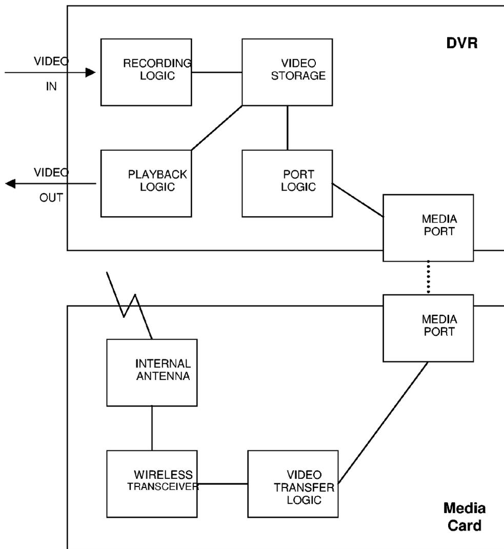
FIG. 2: Block Diagram of a DVR with External Wireless Transceiver
