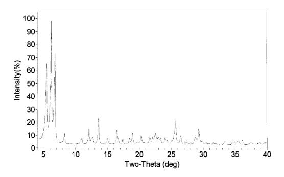
FIGURE 3  $\label{eq:X-ray} \mbox{ X-ray diffraction pattern of calcined ITQ-40 measured with $CuK$$$\alpha$ radiation.}$
