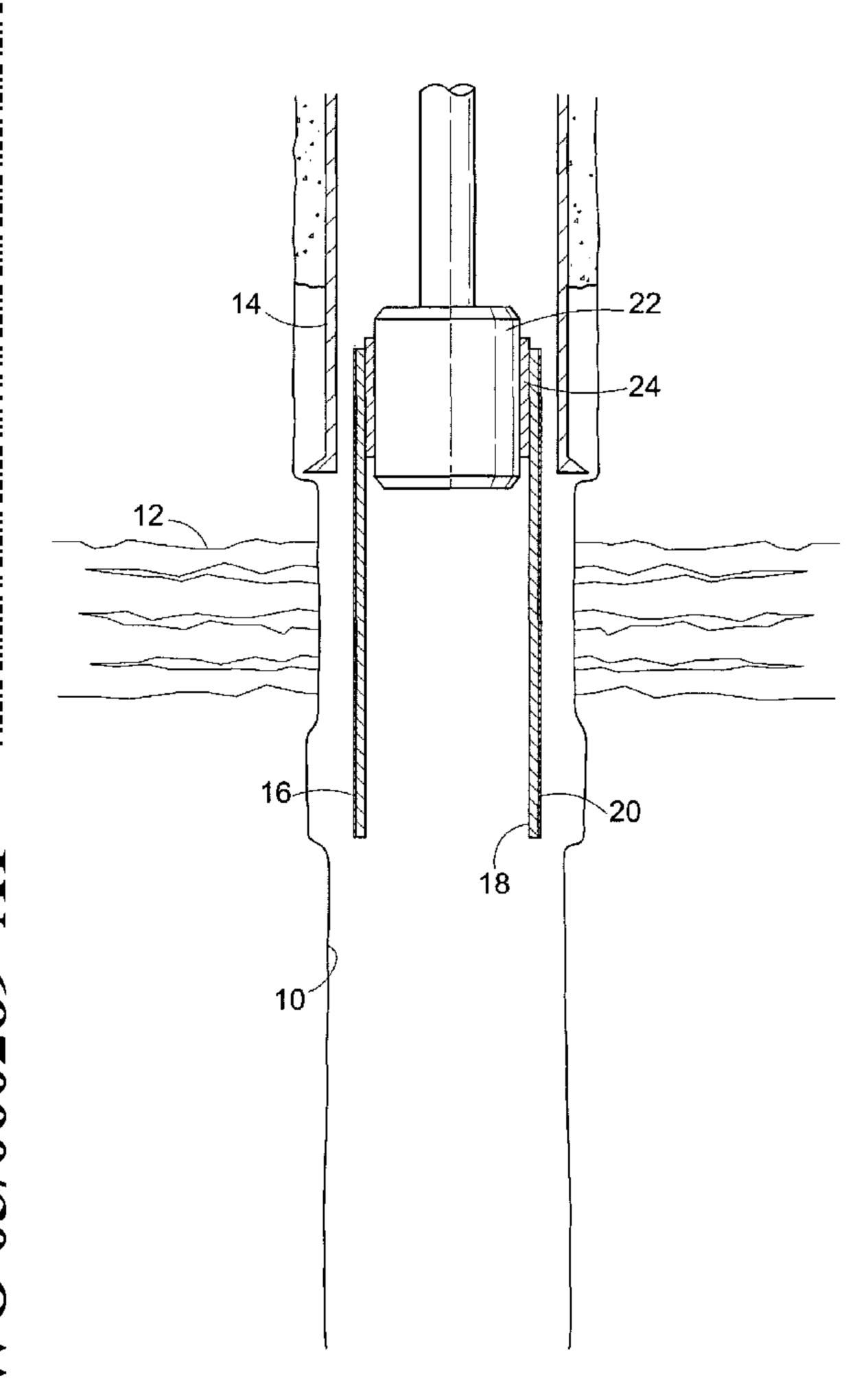
(57) Abstract: A method of isolating a section of a drilled bore (10) containing a problem zone (12) comprises: providing a section of tubing (16); locating the tubing in the section of the bore; and expanding the tubing and forming at least an outer portion (20) of the tubing to conform to irregularities in the bore wall, to isolate the problem zone. The tubing may feature a formable outer section (20), and the expansion of the tubing may be achieved using a compliant rotary expander.
