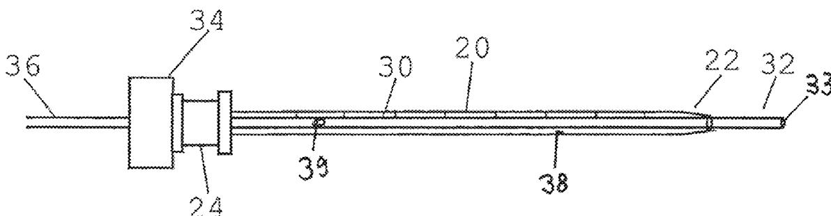
position the distal end of the inner catheter protrudes from the distal end of the catheter sleeve with a pre-defined length which has the outlet opening.
