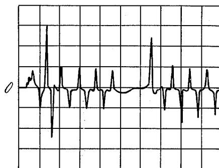
Current Through 35 Mil Spark Gap In Air Vert.-0.5A/Div. Horiz.-50 \mu s/Div.
