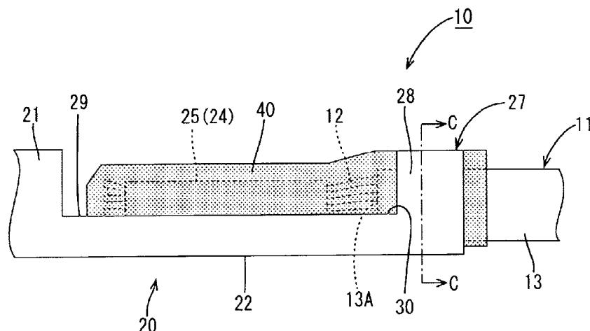
holding portion **27** configured to hold the water stop portion **40** by being held in close contact with an outer surface side of the water stop portion **40**.
