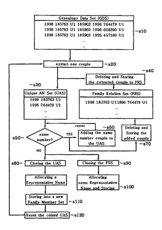
(57) Abstract: The present invention discloses a method for fast searching a genealogical tree among patents recorded in a patent database and displaying the searched results. In details, the present invention extracts the patents having fields containing genealogical tree information from a patent database and makes the patent numbers in the same format and deletes the repeated paren patents and finally generates family relation sets and family member sets to generate the genealogical tree.
