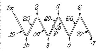
(57) Abstract: The present invention is directed to a multifilament yarn formed at least in part from filaments having cross-sectional zig-zag or double "W" shape with a 180 degree axis of symmetry. The filaments have a denier per filament generally in the range of about 0.1 to about 4.0. Fabrics made from yarns formed with the filaments have high moisture wicking, soft hand, and silk-like lustrous appearance.
