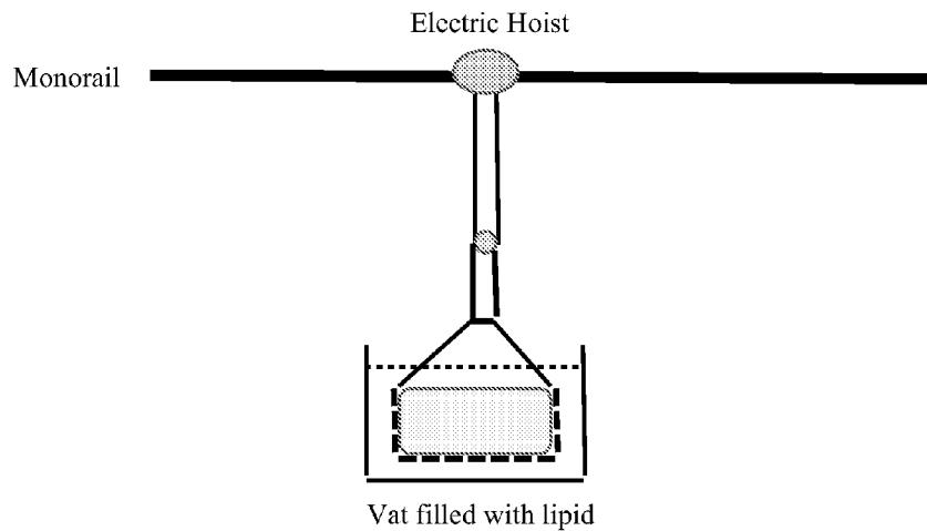
Hay bale fully immersed in lipid. Immersion time is provided to achieve the proper quantity of lipid absorption. The hay bale is supported by a perforated metal basket connected to the ho
