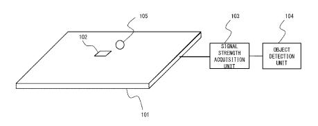
(three or more values of) signal strength of the read signal and physical characteristics of the object to be detected.
