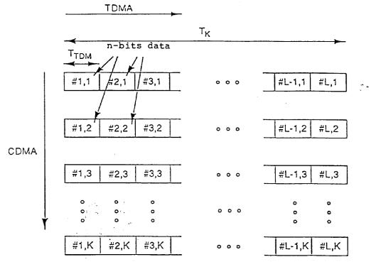
L TDMA-users K CDMA-users  $T_{K}$  = length of frame  $T_{TDM}$  =length of time slot
