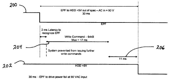
System recognizes EPF – stops issuing write commands
