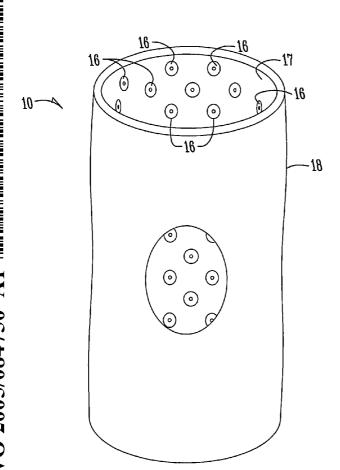
(57) Abstract: A device (10) for applying a therapeutic electrical field to a user's body includes an electroactive material (18) shaped for application to a user body to provide a therapeutic electric field in response to pressure applied to the electroactive material and one or more electrodes (16) integrated into the electroactive material and disposed along an inner surface (17) of the electroactive material for delivering the therapeutic electric field to the user's body.
