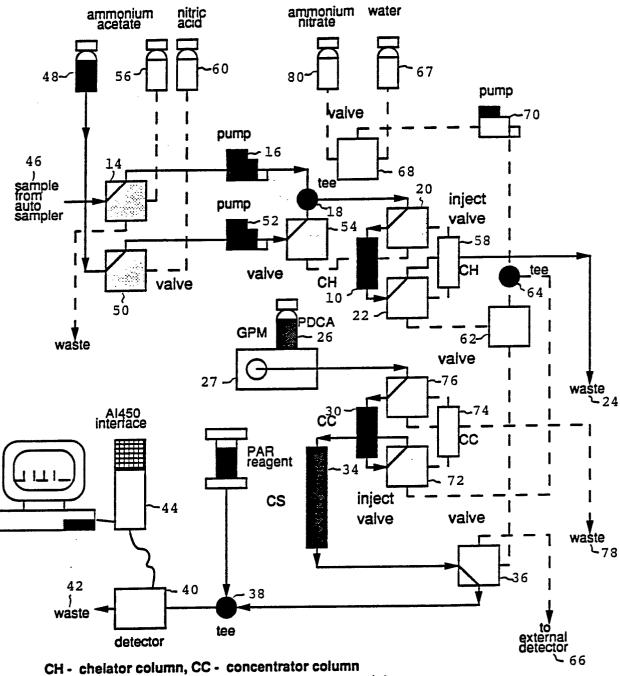
CH - cheiator column, CC - concentrator column CS - analytical column, GPM - gradient pump module
