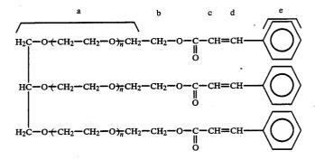
represented by the formula (I), the low molecular weight polyethylene glycol (a), the high molecular weight polyethylene oxide (b), the alkali metal or ammonium salt (c) and a sensitizer are dissolved in a sol- 45 vent such as acetonitrile, acetone, ethanol or tetrahydrofuran, thereby preparing a homogeneous solution. The solution is then cast on a substrate and after substantial removal of the solvent, is exposed to ultraviolet 50 rays to cure the resultant film.
