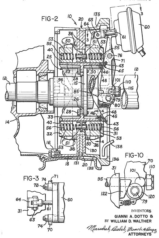
DISC BRAKE AND ACTUATING MEANS THEREFOR
