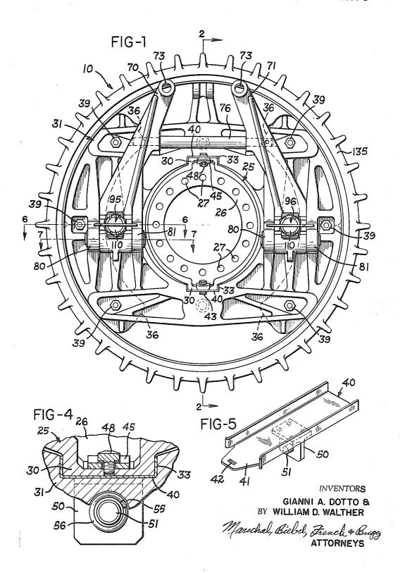
DISC BRAKE AND ACTUATING MEANS THEREFOR
