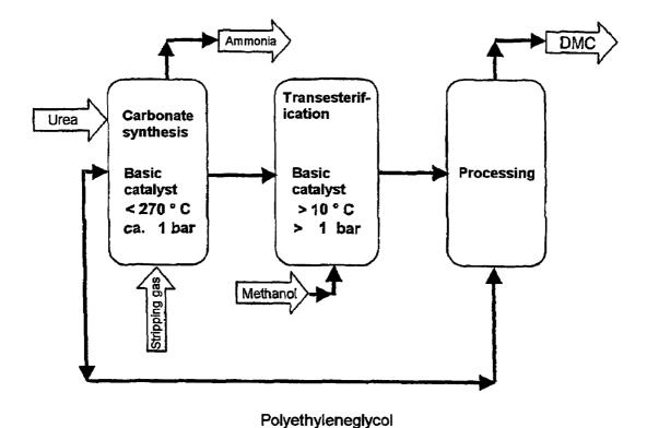
Fig. 1: Example of an engineering arrangement of method for manufacturing organic carbonates, for example DMC manufacture
