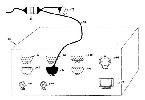
(57) Abstract: Remote monitoring and control of a motorized vehicle (10) is performed using a communications and control hub (46) connected directly to an onboard diagnostic port (44) of the vehicle. An auxiliary onboard diagnostic port (78) is provided to permit technicians to perform diagnostics on the vehicle. All vehicle monitoring and control is effected without an auxiliary wiring harness. The communications control hub is particularly useful for fleet management and dispatch systems.
