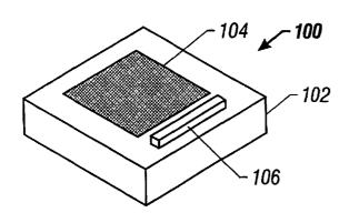
(57) Abstract: A hybrid detector (100) or imager includes two substrates (102, 106) fabricated under incompatible processes. An array of detectors (104), such as charged-coupled devices, are formed on the first substrate using a CCD fabrication process, such as a buried channel or peristaltic process. One or more charge-converting amplifiers (114) are formed on a second substrate using a CMOS fabrication process. The two substrates are then bonded together to form a hybrid detector.
