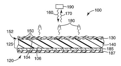
(57) Abstract: The application is directed to a flexible polymer substrate (100) for use in surface enhanced Raman spectroscopy (SERS) and surface plasmon resonance (SPR) measurements. The substrate comprises a polymer film (125) with nanostructured features (152) embosed on one surface and covered with a metallised layer (130), made from gold, silver etc., to produce a SERSactive surface. A method of manufacturing the device is described and applications include DNA sensing.
