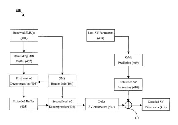
FIG. 4 SMS PROCESSING AT CLIENT DEVICE
