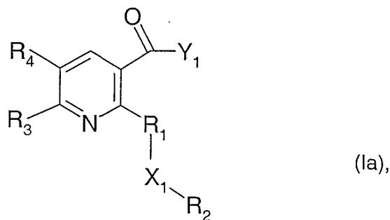
in which R<sub>1</sub>, R<sub>2</sub>, R<sub>3</sub>, R<sub>4</sub>, and X<sub>1</sub> are as defined above and Y<sub>1</sub> is a leaving group, for example halogen, for example by Claisen condensation, or from the compounds of the formula Ia by reaction with a ketocarboxylic acid salt of the formula VII
