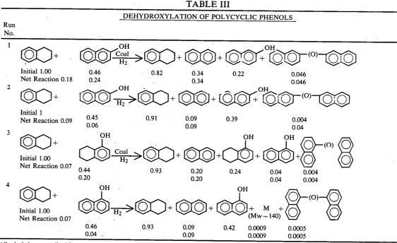
All calculations normalized for 1 mole tetralin in the initial mixture. Methylnaphthalene not included in calculations. All reactions at 800° F., 90 min. Coal (when used) was Burning Star.
