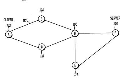
(57) Abstract: Distributed DNS in a wireless communication network comprising broadcasting by a first node a request message to a second node is disclosed. The request message comprises a hostname of the second node. The first node forwards the request message to the second node through intermediate nodes in the wireless communication network and the second node transmits a response message to the first node. The response message comprises a MAC address of the second node.
