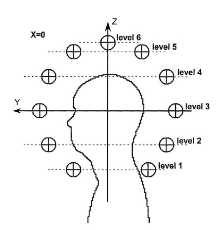
(57) Abstract: An arrav coil to achieve more uniform RF excitation for high field magnetic resonance imaging. In the preferred embodiment, the array coil has a plurality of transmit- composite elements distributed around the object to be imaged. A composite element comprises up three current loops preferably orthogonal to each another. The array coil has the capability to shape the distribution of all three orthogonal components (x, y, and z) of the RF B<sub>1</sub> field.
