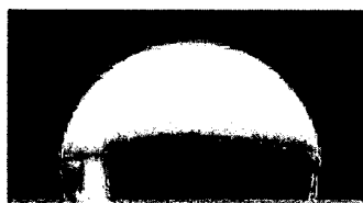
A PTFE SUBSTRATE (NOT TREATED) \theta = 103.9^\circ
