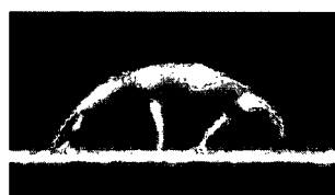
A SUS316 SUBSTRATE (NOT TREATED) \theta = 75.5^\circ
