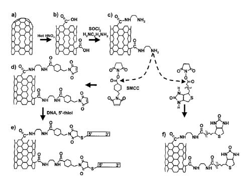
(57) Abstract: This invention provides surfaces having nanocylinders, such as carbon nanotubes, attached thereto through biomolecular interactions, devices made from assemblies of nanocylinder-modified surfaces, and methods for producing nanocylinder modified surfaces. A variety of biomolecular interactions may be used to attach the nanocylinders to the surfaces, including hybridization of complementary oligonucleotide sequences and receptor-ligand interactions.
