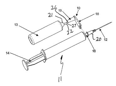
(57) Abstract: A clip (10) to releasably engage an ampoule (13) and syringe (11). The clip (10) includes an ampoule engaging portion (19) and a syringe engaging portion in the form of a recess (17). The ampoule engaging portion (19) is formed of resilient material so that upon insertion in the neck (21) of the ampoule (13) the portion (19) is compressed so as to aid in engagement with the ampoule (13).
