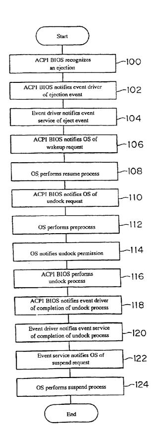
SYSTEM FOR NOTIFYING OPERATING SYSTEM OF ADDITIONAL EVENT FOR RESTORING SUSPEND MODE AFTER A HARDWARE DEVICE EVENT SWITCHES COMPUTER TO NORMAL MODE
