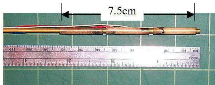
Fig 10 Three-element ultrasound applicator for the treatment of uterus
