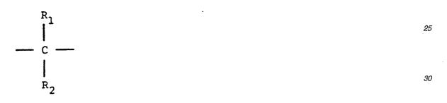
wherein  $R_1$  and  $R_2$  are independently hydrogen, aryl of 6 to 12 carbon atoms,  $C_1$  to  $C_9$  alkyl or form an alicyclic ring of 3 to 9 carbon atoms, a is an integer of 0 to 4 and n is independently an integer of 1 to 3, bisphenol J has the structure:
