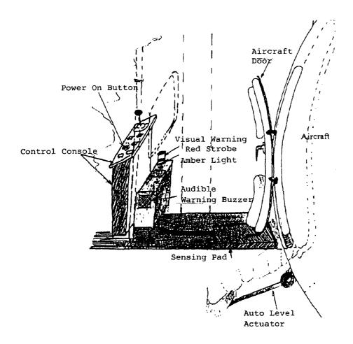
Figure 4 Operational View of Control Console and Panel
