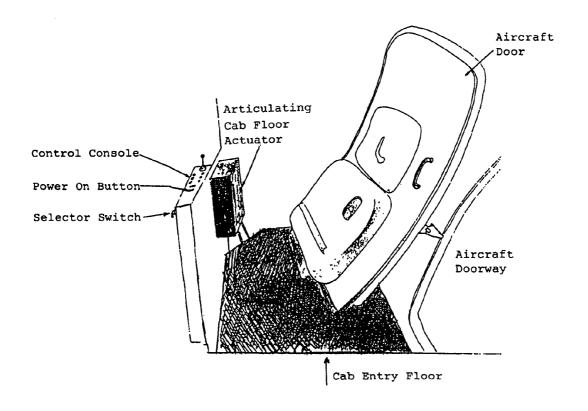
Figure 2 Existing PLB Installation As Currently Configured
