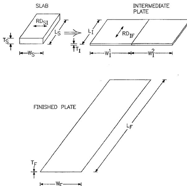
(57) Abstract: A method of making metal plates as well as sputtering targets is described. In addition, products made by the process of the present invention are further described. The present invention preferably provides a product with reduced or minimized marbling on the surface of the metal product which has a multitude of benefits.
