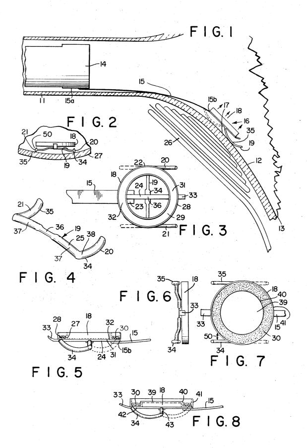
This invention relates to an improved getter assembly and more particularly to an improved channel ring getter assembly adapted for mounting in a television picture tube against a wall thereof without danger of damaging said wall during insertion of the device into the tube or during flashing of the getter material and without danger of entanglement with other adjacent getter assemblies.
