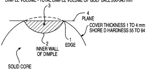
DEFORMATION AMT. 2.3 TO 3.5 mm JIS-C HARDNESS OF 50 TO 85 JIS-C HARDNESS DISTRIBUTION WITHIN 5
