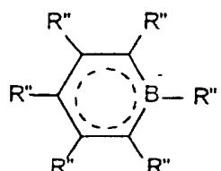
wherein each R'' is independently selected from the group consisting of hydrocarbyl, silyl, or germyl radicals, 50 each said R'' having up to 20 non-hydrogen atoms, and being optionally substituted with a group containing a Group 15 or 16 element. In complexes involving divalent derivatives of such delocalized  $\pi$ -bonded groups one atom thereof is bonded by means of a covalent bond or a covalently bonded divalent group to another atom of the complex thereby forming a bridged system.
