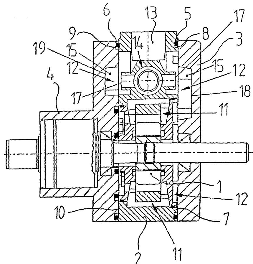
(57) Abstract: The invention relates to a pump for delivering a fluid, especially to a vane-cell pump, comprising a delivery device (1) housed in a housing (2), a supply channel (13) for the fluid that is formed in the housing (2) and that extends into the intake zone of the delivery device (1) and leads to a jet chamber (15) disposed upstream of the delivery device (1), and an injector device (14) for delivering the fluid.
