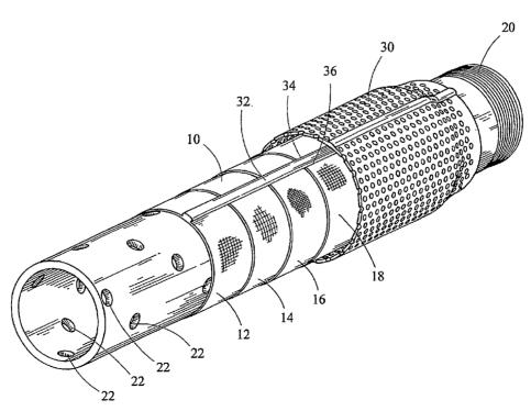
(57) Abstract: A particle control screen includes a support layer. A first filter layer is disposed around the support layer. A second filter layer is disposed around the first filter layer. A third filter layer is disposed around the second filter layer. Each of the filter layers has a pore size. The pore size of the third filter layer is greater than the pore size of the second filter layer. The pore size of the second filter layer is greater than the pore size of the first filter layer.
