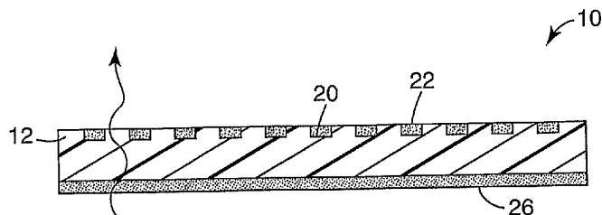
(57) Abstract: The present application is related to substrates having light transmitting areas and light shielding areas. The application discloses methods of manufacturing the substrates, including modifying a light shielding layer to contact to a structured surface.
