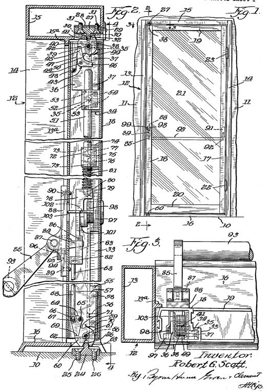
LOCKING MECHANISM AND PANIC ACTUATING DEVICE
