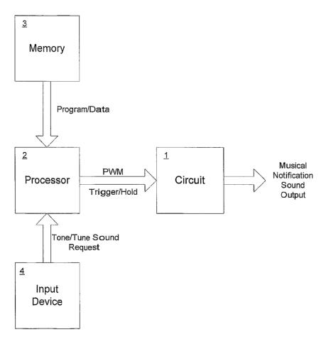
(57) Abstract: A flexible audio tone-generating device for use in a consumer appliance. The device generates pleasing musical tones. The device uses two outputs of a software-executing processor utilizing stored tone data associated with status events of the appliance to drive a tone circuit for outputting a melody using the tones to notify the user of the existence of one of the status events.
