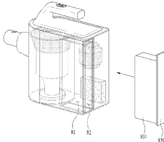
provided to supply power to the fan, and a handle part including a handle base coupled to a top side of the first housing and a handle body connected to the handle base.
