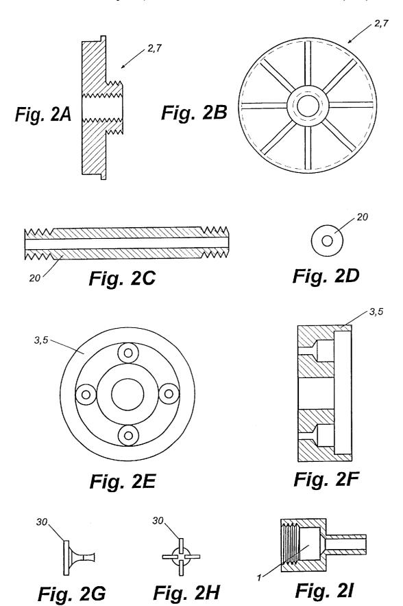
TRANSVERSE CROSS SECTION OF CYLINDRICAL ROD THROUGH WHICH GAS PASSES THROUGH WHILE BEING HEATED
