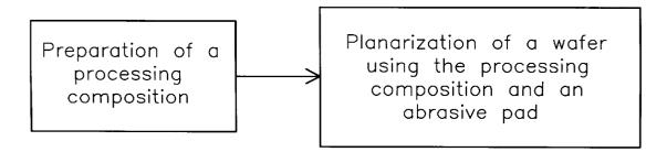
Planarization Using a Processing Composition
