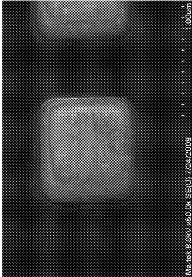
Post-SFP Sample: Etched by using XeF2 with pretreatment of Ta oxide removal
