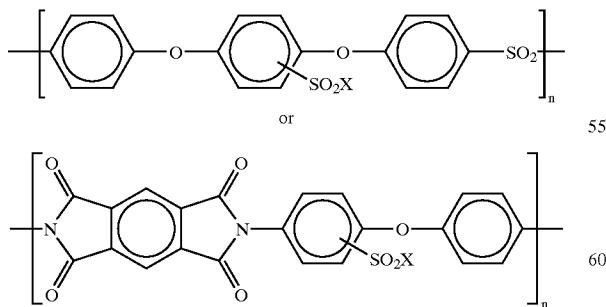
Once obtained, the copolymer containing the above precursors is molded, for example in the form of sheets, and converted into an ionic form through hydrolysis, to give species of the sulfonate or carboxylate type. The cation
