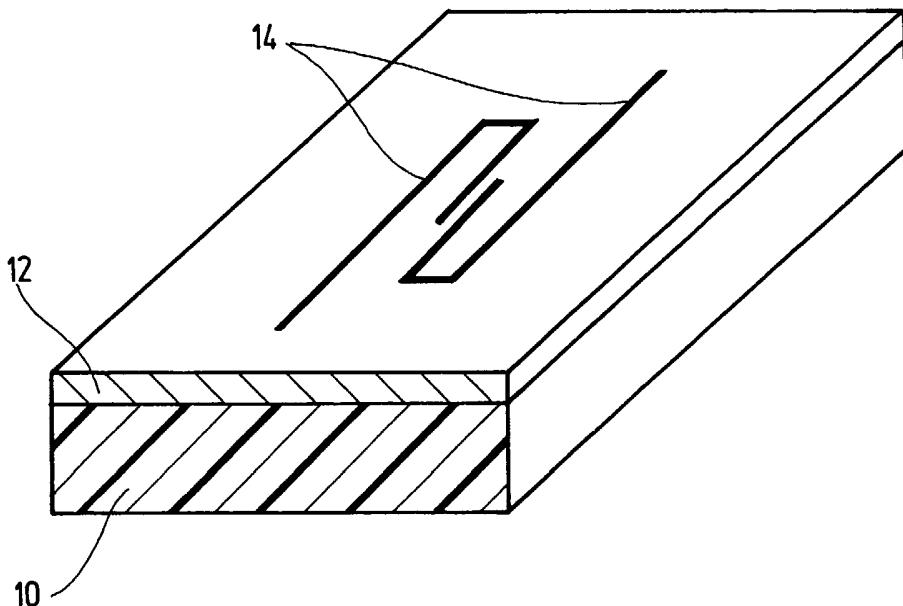
(57) Abstract: The invention relates to a method for the production of an insulating substrate provided with a layer electrode, in particular for an analytical test strip. A combination of the following method steps is disclosed:- the layer electrode (14) is formed as a structured surface pattern on the substrate (10) and the hydrophilicity of a cover layer (12) on the substrate (10) is increased by a chemical or physical surface treatment.
