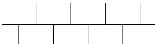
[0046] Polypropylene having this type of chain configuration is called syndiotactic polypropylene, or sPP.
